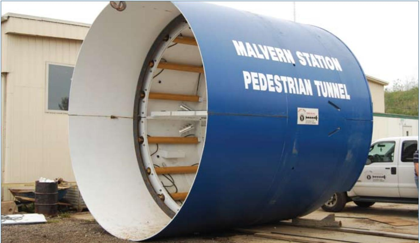
The 15-ft diameter hydraulic shield was constructed by Turn-Key Tunneling in conjunction with Tunnel Shields & Equipment Inc.
